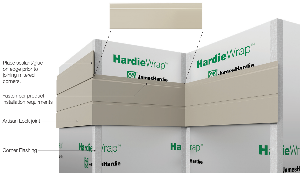
Figure 11. Mitered internal and external corners for Artisan siding with Lock Joint system.
