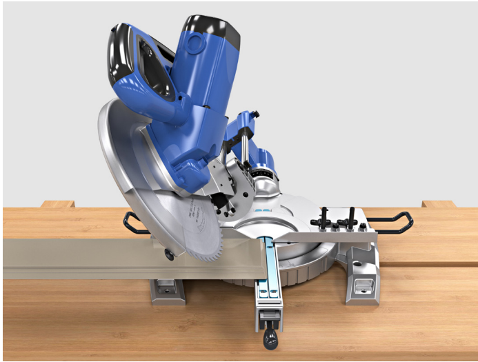
Figure 9. Left-hand miter = Feed board plank face down with top edge away from fence.
