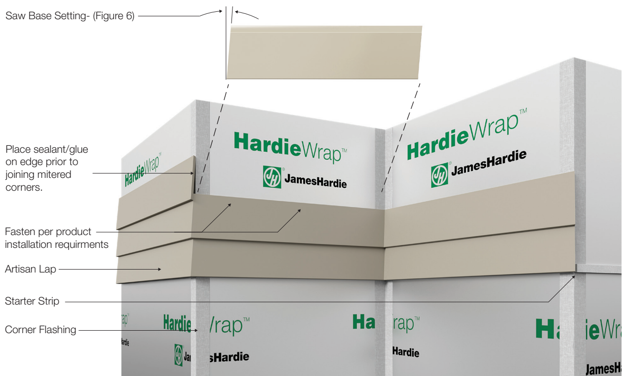
Figure 8. Artisan Lap siding installation with mitered internal and external corners.
